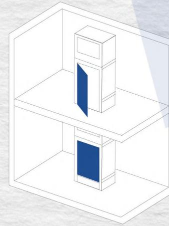
Elevator can be installed in the floor opening
